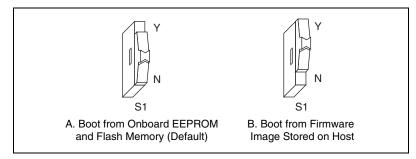
Figure C-1. Firmware Recovery Operation
